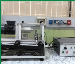
Slack checking device It is used in mechanical design to calculate the number of fatigue cycles a metal can withstand under applied load.
