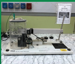
Creep testing machine This device provides mechanical properties of metals and non-metals by applying a constant load and extracting the relationship between strain and time.
