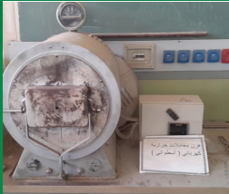
Electric furnace for thermal processing labs Conducting engineering inspections on metals following heat
