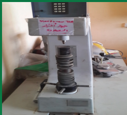
Hardness testing machine Calculating hardness values for metals using Brinell and Vickers methods.
