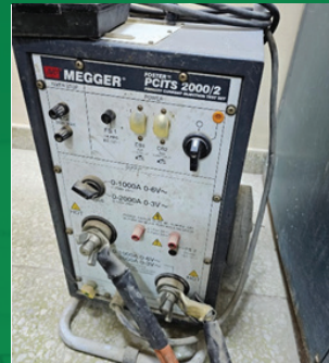
Testing circuit breakers (trip time testing + contact resistance testing)
