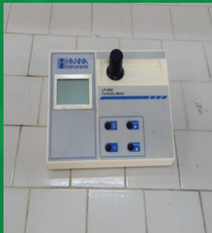
A device to measure fine turbidity of the table
