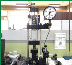
Tensile testing machine A device that provides mechanical properties of both metals and non-metals, with a measurement range of up to 20 kiloNewtons.
