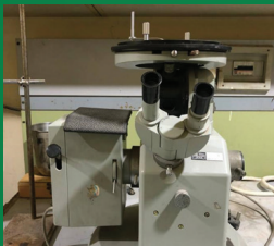
Optical microscope for examining the microstructure of metals It's a type of microscope that uses light and a lens system to generate magnified images of metal surfaces. It is used to examine metals and engineering materials.
